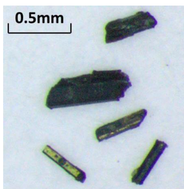
Figure 1. Representative single crystals of \text{Ba}_8\text{Al}_2\text{IrO}_{14} .
